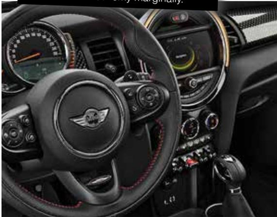
The iconic central instrument now has a four-line TFT display as standard or an optional colour screen showing vehicle functions, infotainment, navigation and Mini Connected services.
