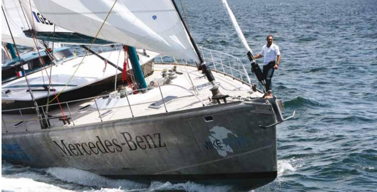
The Pangaea is 35 metres in length and has berths for 30 people. She is powered either by sail or by Mercedes-Benz diesel engines. Solar panels provide power for state-of-the-art information technologies.
